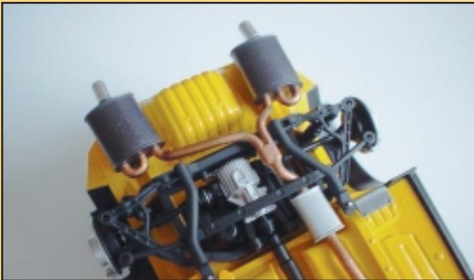
**6** This is how rear suspension looks when assembled. Interesting thing is that a bar secures the whole thing after the exhaust was installed. In this picture you can see that drive shaft is a two-piece part.
