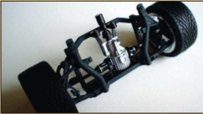
**4** Here is the rear suspension. Brilliant Tamiya engineering recreates the real thing perfectly! I wish the drive shaft was a whole piece, though! I applied some Bare-Metal Foil to simulate boot clamps.
